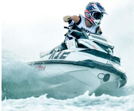
The engine provides power to the Jet-Pump which sucks in water through an open grate at the bottom of the jet-ski hull, pressurizes the water by an inner turbo system and then expels it out at high speed through the nozzle at the rear of the ski. This nozzle is directional and thereby provides the steering ability. The moment a jet-ski is started, the jet pump is functional and will start to propel the jet-ski forward or backwards according to the position of the gear lever.
